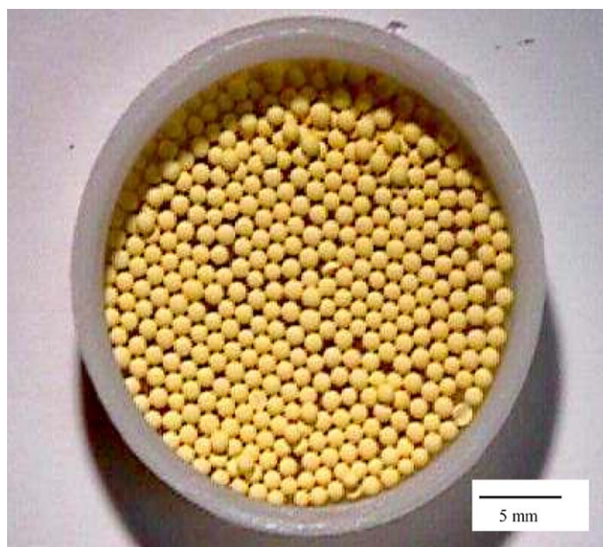
Fig. 8. Dry \text{UO}_3 microsphere.
